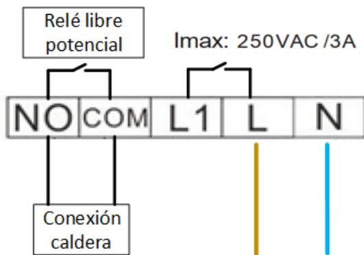
CABLEADO A CALDERA Y CABEZAL TERMOELÉCTRICO
